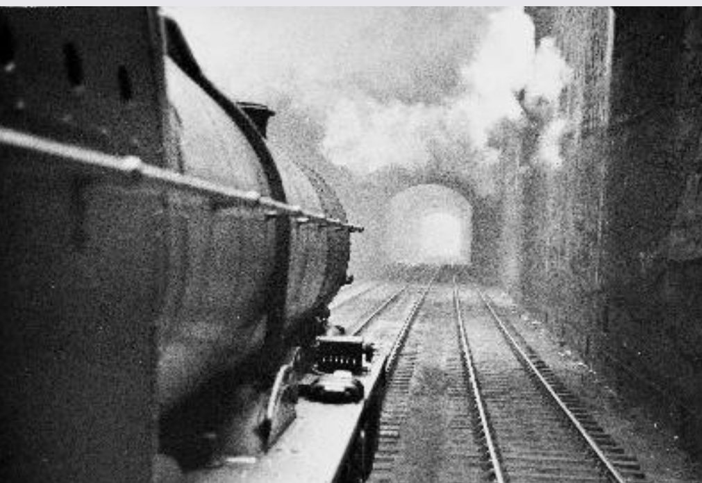
'A 'Princess Royal' 4-6-2 pounds up the 1 in 93 gradient from Lime Street in the vertical rock-sided cutting through the city of Liverpool.
