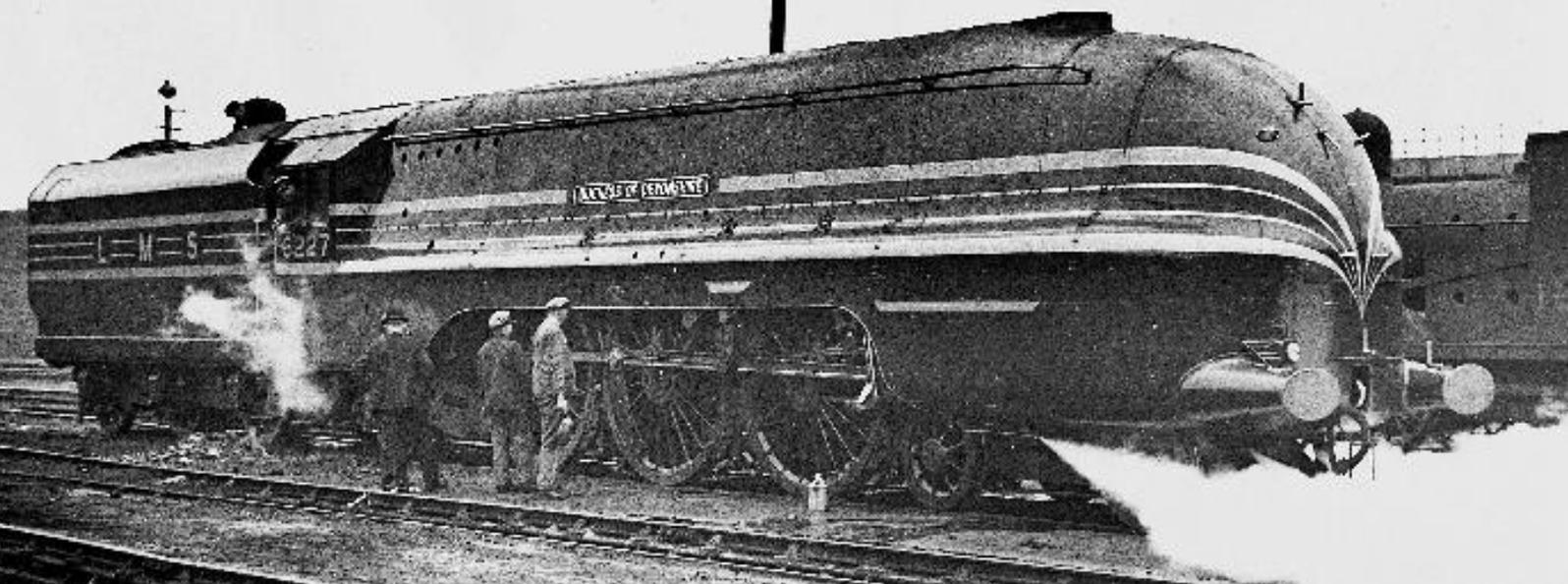
New 'Princess Coronation' Pacific No.6227 *Duchess of Devonshire* is checked over at Edge Hill depot on 24th June 1938 before working the 12 noon Liverpool Lime Street–Plymouth as far as Shrewsbury on a running-in turn under the supervision of the bowler-hatted inspector. Note the special design of 'streamlined' headlamp.
