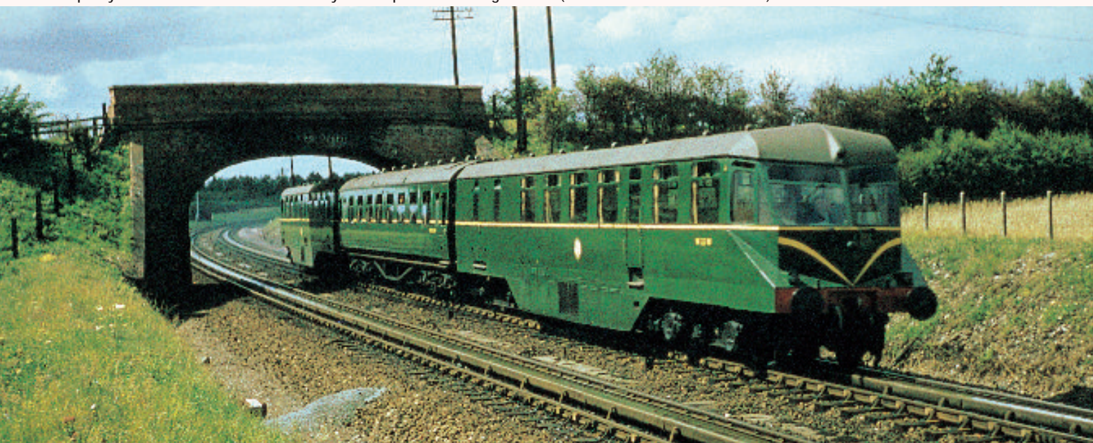
BELOW: The logical next step was to produce a twin-car unit and the Great Western introduced two such pairs in 1941/2, Nos.35/36 and 37/38. These featured a buffet counter and were intended to replace single cars on the Birmingham–Cardiff run but in fact were so successful in attracting passengers that conventional steam trains of greater capacity had to take over the service! They were capable of running with
