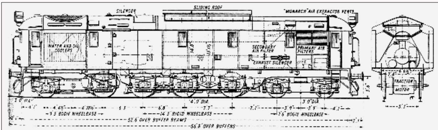
The diagram for the Armstrong, Whitworth 1,200hp (Sulzer 8LD34 Type engine). The post-war English Electric 1,600hp main line locomotives for Egypt of the (1A) 'Do (A1)' type were almost certainly influenced by this design. Note the positioning of metal 'N.W.R.' letters on the side sheeting, something adopted on No.10000 — 'L.M.S.' in 1947. (Author's Collection)
