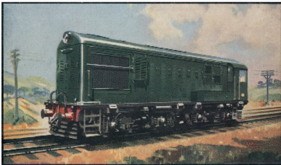
The 100-ton Diesel Electric Locomotive, No. 200, built by the Vulcan Foundry Limited in conjunction with The English Electric Company Limited, at Newton-le-Willows, Lancs., in 1957.
